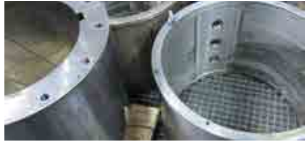
Bushings before repair
