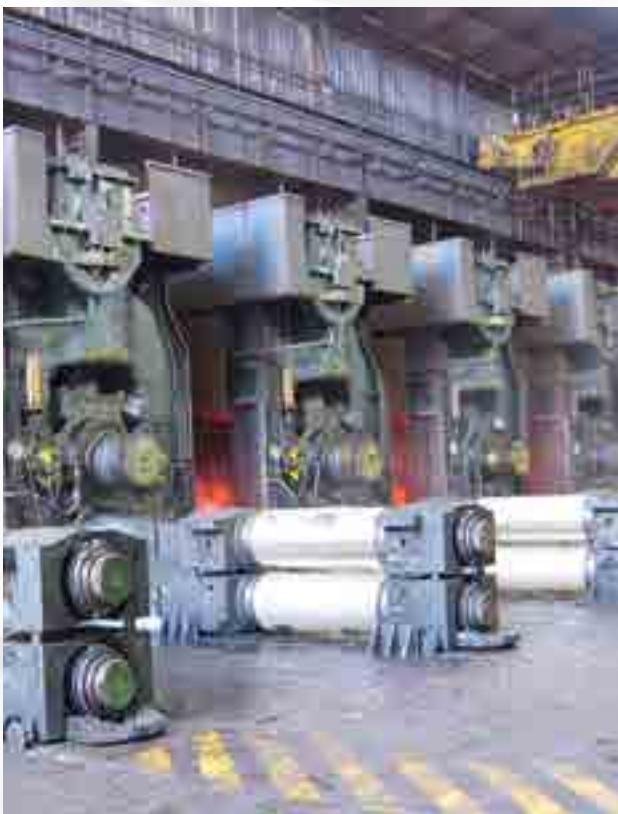
Hot strip finishing mill
